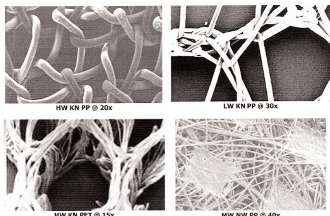
Figure 1: Overview of knitted and non-woven non-barrier surgical mesh structures at various magnifications.
